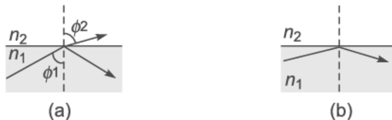
Fig 3.1 (a) For a ray incident on a rarer medium ( n_2 < n_1 ), the angle of refraction is greater than the angle of incidence, (b) if the angle of incidence is greater than critical angle, it will undergo total internal reflection.
