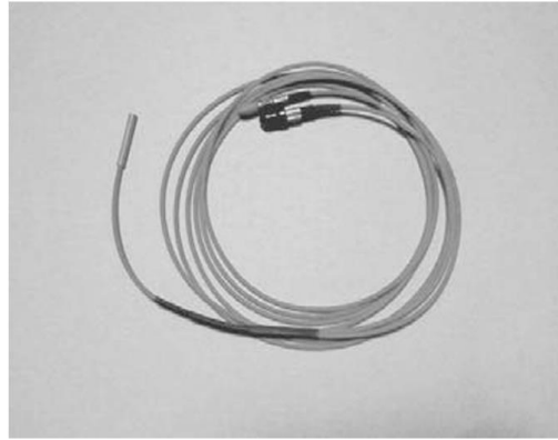
Fig 3.9 Typical cabled probe used for displacement measurement
